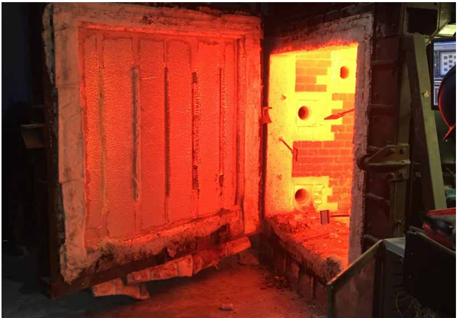
Furnace with vertical linear seals after resistance to fire test acc. EN 1366-4.
