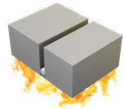
3. Single seal, exposed side
