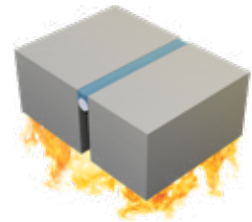
2. Single seal, unexposed side
