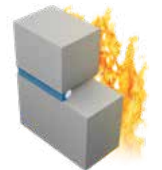
2. Single seal, unexposed side
