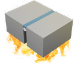
2. Single seal, unexposed side
