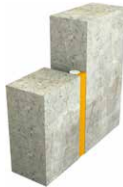
PE backer rod and fire resistant sealant
